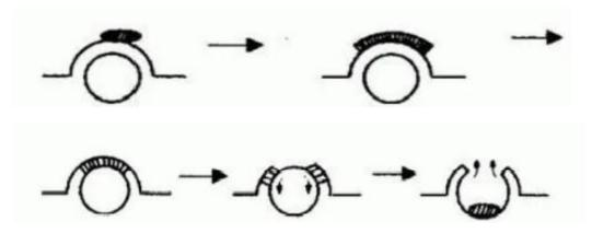
1. Contacting with defoamer→2. Molecule diffusion→3. Molecules enter into the bubble film→4. Bubble film thinning→5.Bursting
